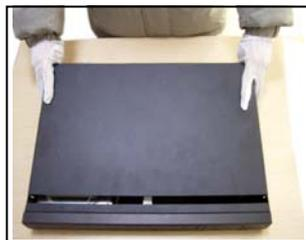
② disassemble the crust
